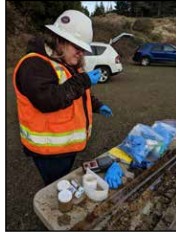
An environmental compliance contractor attempts to detect the presence of petroleum or other odorous chemical contamination from soil before bagging and labeling samples for formal laboratory analysis. Photographed by Adrienne Kirk, 2018.
