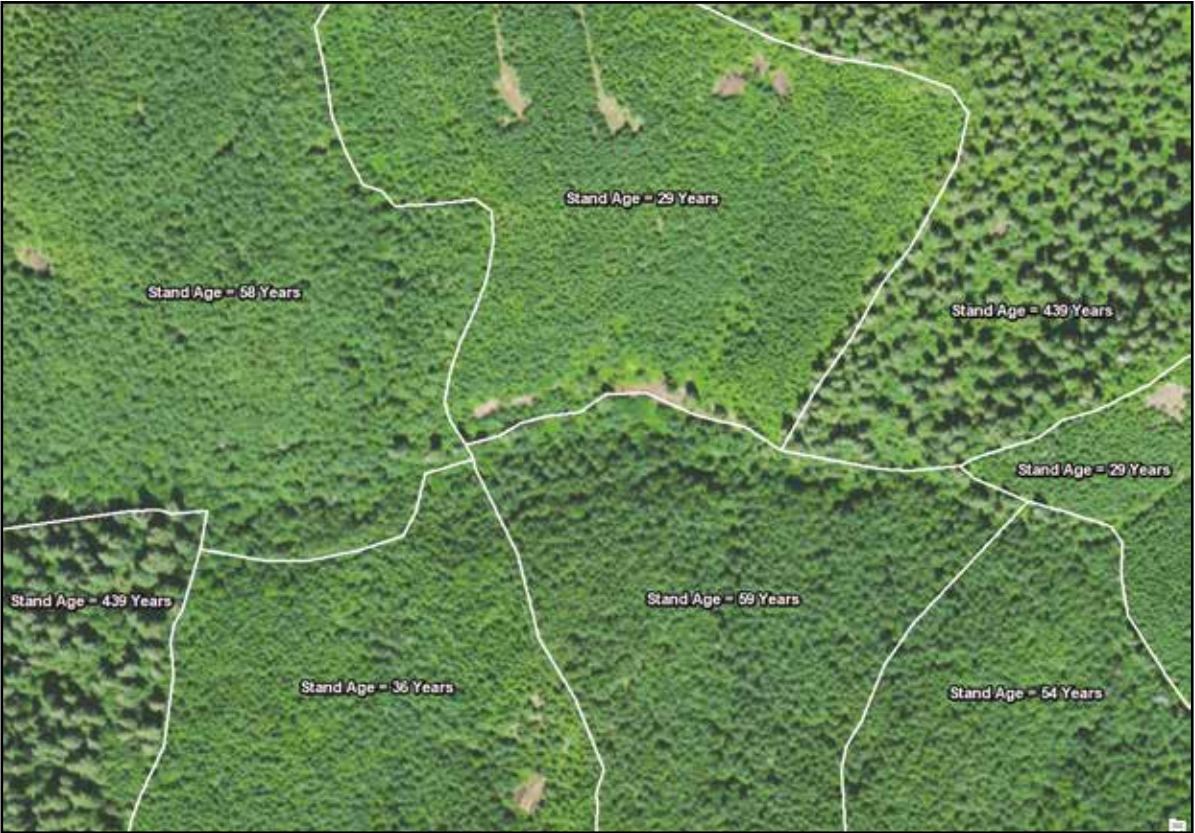
Photo 1: Traditional aerial photos such as this can be used to delineate stands containing trees of similar heights. The limitation of aerial photography is apparent, as the 36-year-old stand and the 59-year-old stand look similar on the aerial photo.
